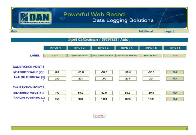
For the input being calibrated, insert into CALIBRATION POINT 1, the actual MEASURED VALUE (0.0) and into the ANALOGUE TO DIGITAL box the binary data as noted from the search of data above.
