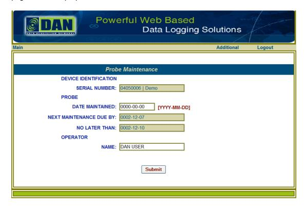
The 'Probe Maintenance' page is intended to be used as a manually maintained reporting facility. Each time probes are cleaned, the date is entered into the 'DATE MAINTAINED:' window. The next scheduled date for maintenance will be calculated and displayed. A second date will also be calculated representing the latest date recommended. (Recommended periods are automatically based on a fixed weekly cycle)
